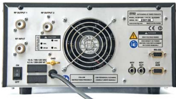
Figure 4 — The rear panel, showing the cooling fan and available connections.
