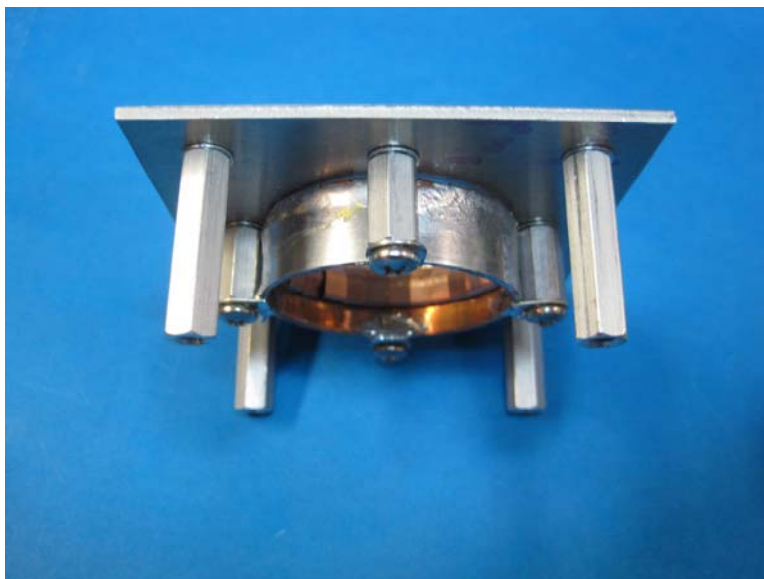
Top Half of Socket with New Short Screws
