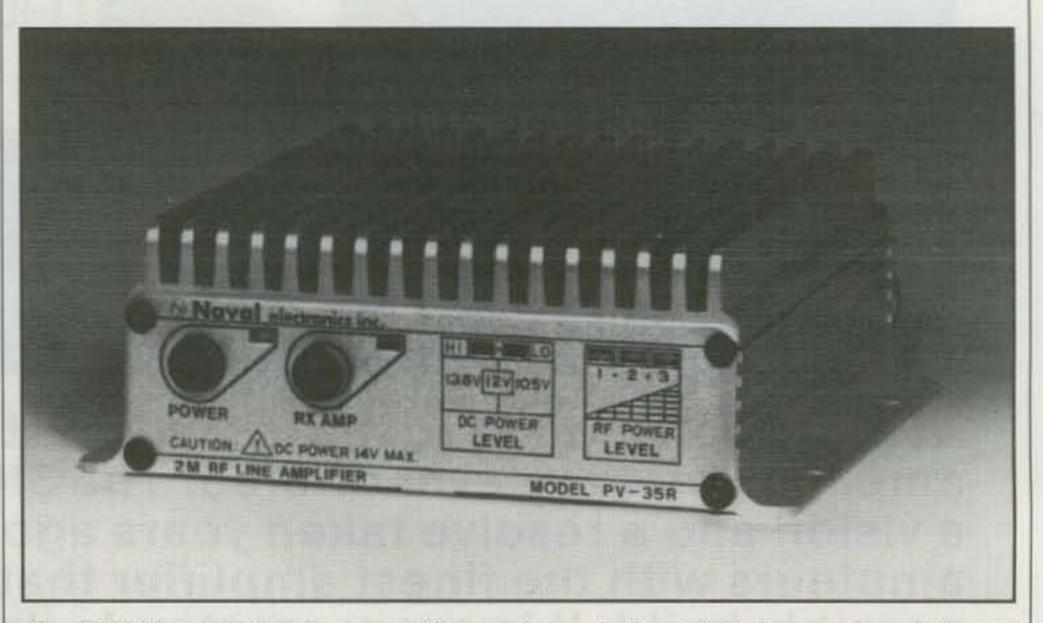
The PV-35B presents a neat amplifier package. At the right is the power switch, and to its right is the receiver amplifier. The DC power levels are displayed via LEDs, as are the output levels.
