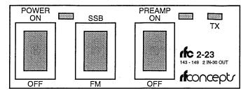
**POWER**: This switch activates the power amplifier section.
