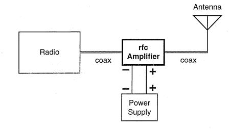
equivalent coax is recommended. For best performance, the antenna should be adjusted for an SWR of less than 2:1.
