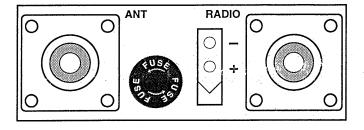
**ANT**: Antenna connection. Looking from the back, this is the left-hand coax connector. CAUTION: Do not connect your transceiver to the amplifier "ANT" port. Damage to amp could occur.
