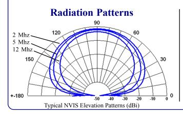
Inverted Vee ..... Combination Horizontal and Vertical
