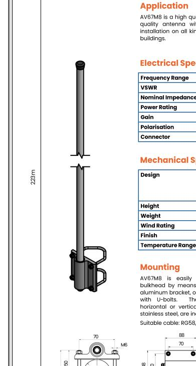
AV67M8 is a high quality dipole antenna designed for marine VHF. It is a high quality antenna with a durable construction and a beautiful finish for installation on all kinds of vessels. The base also makes it easy to install on
