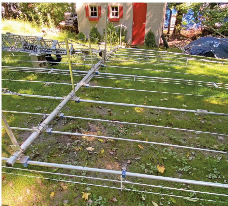
Figure 5 — The assembled antenna on the tower TiltPlate lowered at ground level.
