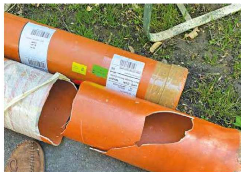
Figure 7 — The antenna packaging tube that arrived damaged and that was taped together.
