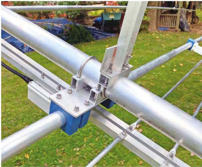
Figure 8 — The elements mounting point with the plastic standoffs.
