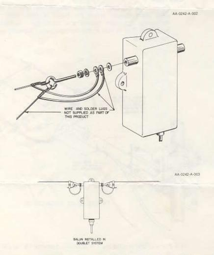
**NOTE:** An ohmmeter check of the balun at all points will show a DC short. This is normal! This is not a short with respect to RF energy at the balun's design frequency.
