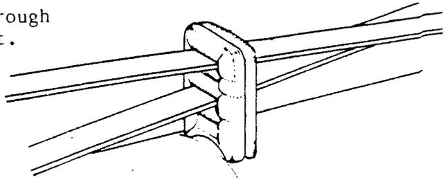
C. Attach balun clip to top center of element #3 with a #6 x 3/8 sheet metal screw. Place balun in clip, connector pointing to boom center. Keep balun terminals as close as possible to feedpoints but a minimum of 3/8" from balun clip. (See last page for details on making your own coax balun)
