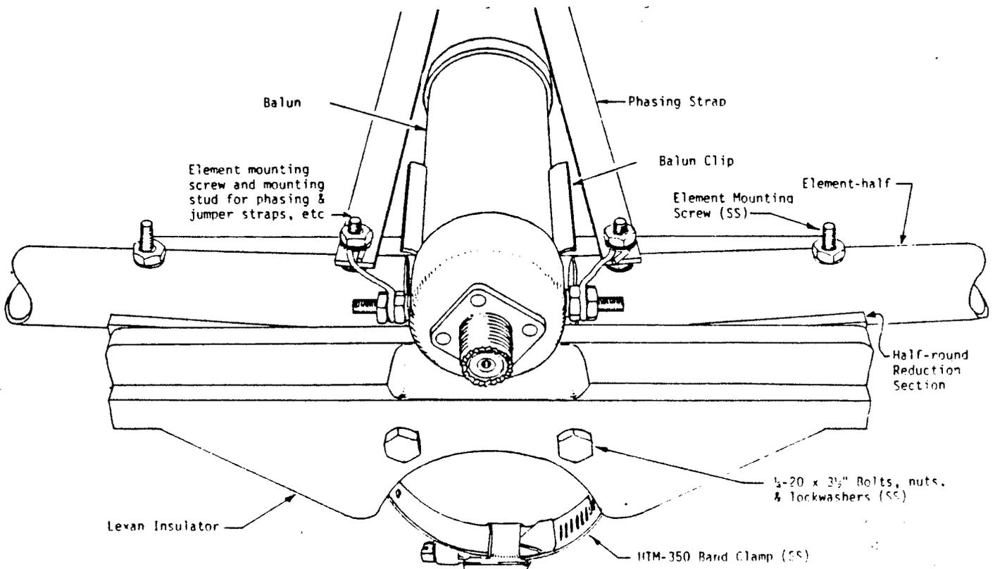
D. Take up any slack in phasing straps by tapping element #3 away from #2. When straps are taut, align element #3 with the rest and tighten clamp.
