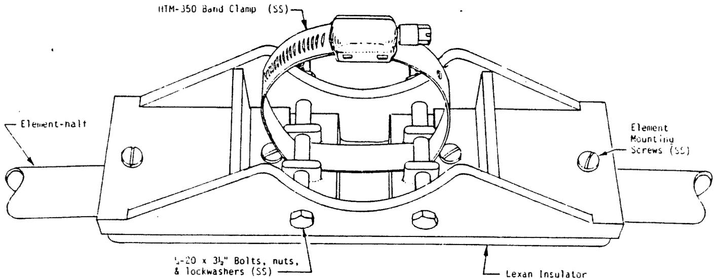
B. The KLM Lexan insulator has been designed to accommodate up to  $1\frac{1}{2}$ " o.d. elements. Antennas using smaller o.d. elements are supplied with half-round reduction sections. These are placed in the two element channels on the top of the insulator with the thicker ends toward center as shown in the drawing below. Prepare all insulators.
