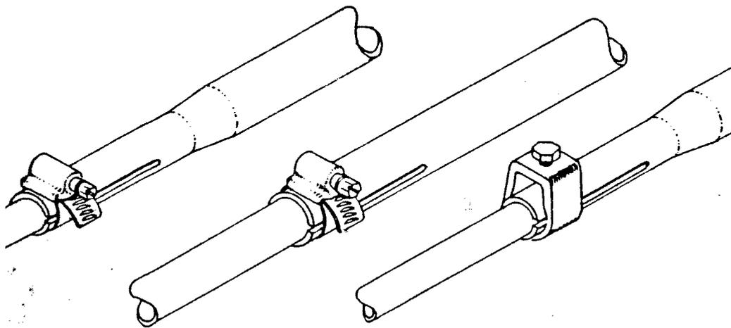
D. The chart below lists the tubing lengths supplied for each element half, the proper band clamp for each overlap, and the correct element half length (adjust the tip section!) Remember to use Penetrox at each overlap and securely tighten clamps until tubing cannot be pulled out or rotated. Pair up element halves as they are completed to avoid mixups.
