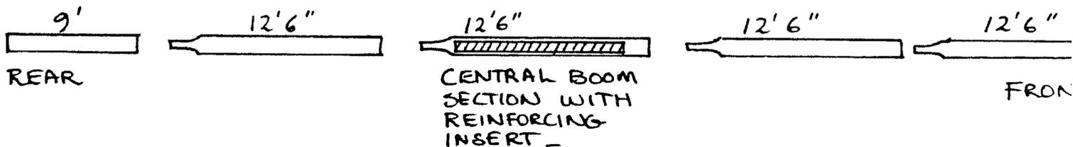
2. One 12' 6" section contains an 11' 6"x 2.85"O.D. reinforcing insert and will be heavier than the others. This section becomes the middle of the boom and provides additional strength in the area of the boom to mast plate.
