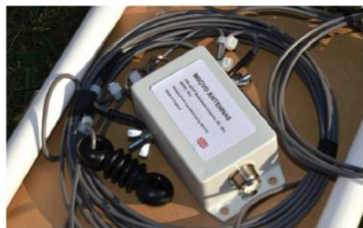
A 4:1 balun of M0CVO's design is added at the feed point.
