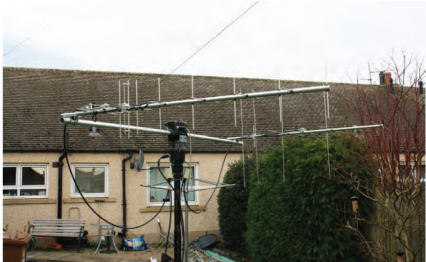
The finished installation, complete with azimuth/elevation rotator.
