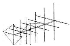
The 12 element Laser 400° is designed to achieve the maximum gain and front-to-back ratio using a Quad reflector and Yagi parasitic elements. There are 6 elements horizontal and 6 elements vertical, all scientifically spaced on a 31' boom. The Laser 400° is second only to the Super Laser 500°. It uses the same top quality design and construction as the larger Laser 500°, but uses a 2" boom.
