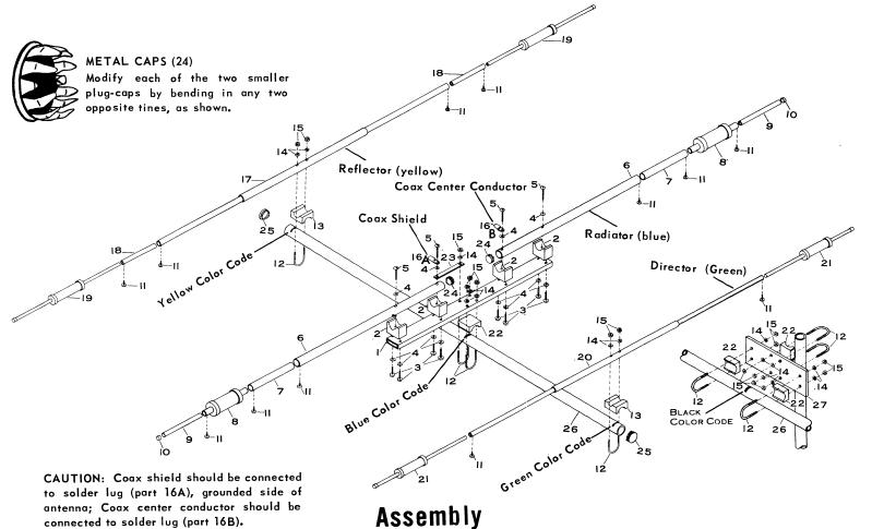
CAUTION: Coil assemblies are color coded on one end only; this color code should always be nearest the boom. Reversal of traps will cause high SWR and other malfunction of beam. The coding on the adjusting holes may be determined from the frequency chart. Adjusting holes do not appear on the reflector trap assembly (yellow) and radiator trap assembly (blue), but on elements sections (parts 18&7).
