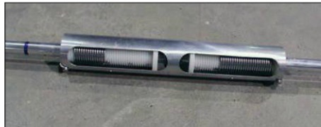
Figure 1 — Cutaway view shows a two-coil trap. The coils and tube capacitance form a resonant circuit, and the 2-inch outer tube is part of an element (usually for 15 meters).
