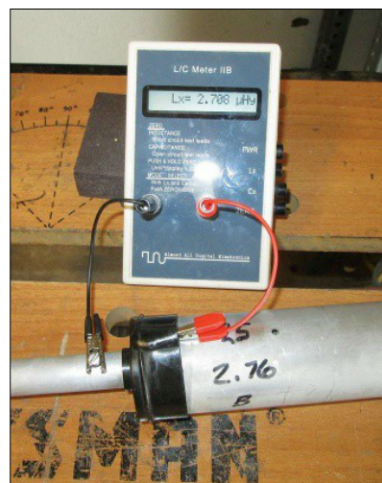
Figure 2 — Connect an LC meter as shown to measure the trap inductance.
