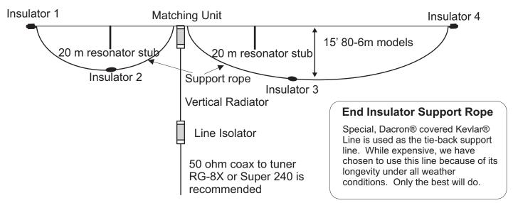
There are several differences between the CAROLINA WINDOM® 80 and the CAROLINA WINDOM® Compact  $80^{\text{TM}}$ . From the diagram above, it is obvious that the new "Compact<sup>TM"</sup> series is much more complex, in that it has 20 meter resonator stubs and it's top elements are folded back toward the matching unit.
