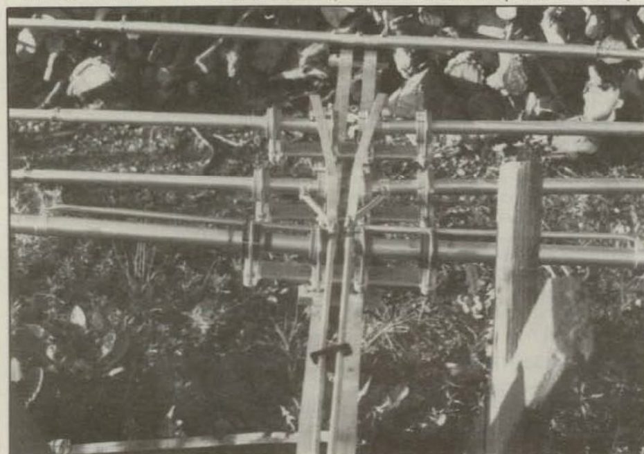
This is the cluster of elements at the front, which is also the feedpoint of the array.
