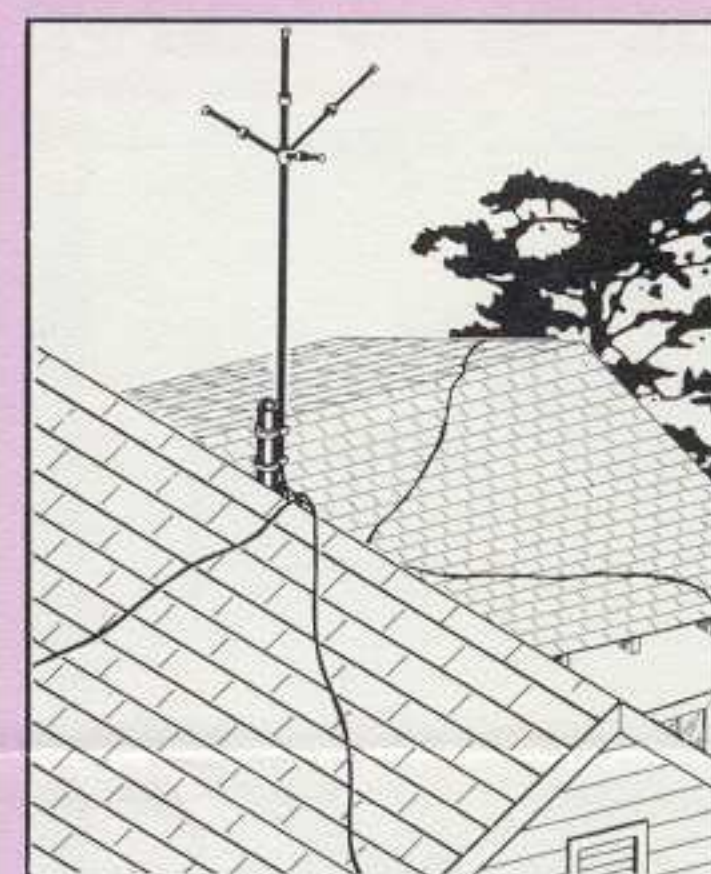
Roof mounted installation with ground radial system.
