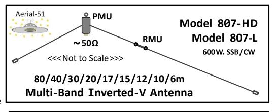
WARNING: The SWR on 60 & 30m is about 10:1 at the feedpoint of the antenna. MAX PWR: 150W on these bands. With some lengths of coax, the SWR may look much better in the shack. However, "at the feedpoint" it is still 10:1 and the ~HIGH VOLTAGE~ caused by running high power on these bands may damage or totally destroy the PMU and/or RMU.
