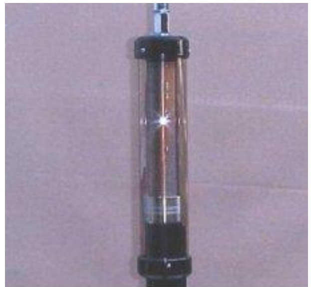
Little Tarheel in 40 meter position with 32" whip
