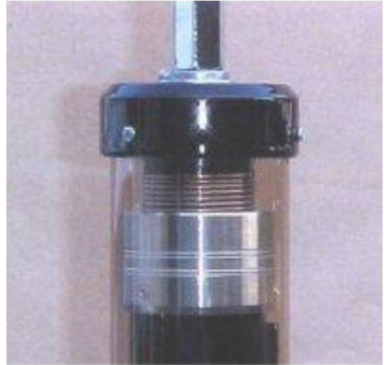
Little Tarheel in 10 meter position with 32" whip
