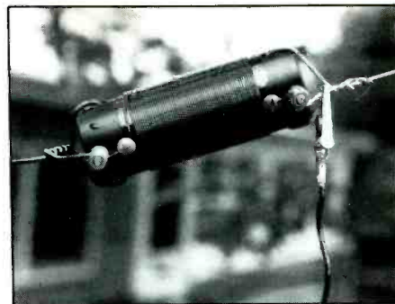
Fig. 4. Clip-on wire for tuning 80M wire to CW portion of band.
