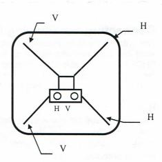
Seen from back of the antenna: right jack is the vertical connector. For adjustment of SWR in vertical plane, bend the left ends of the first director to front or back of the antenna.
