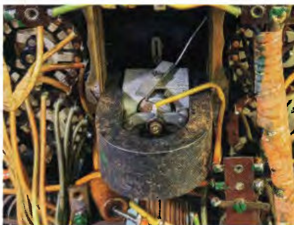
Photo 10: The meter movement is a high-precision instrument, but unfortunately, it's exposed to the inside of the case in the original Valve Tester. So you have to be careful not to contaminate or damage it if you open the unit up. Note the magnetic adjustment tab visible at the back; this gives a 5% or so FSD adjustment range.
