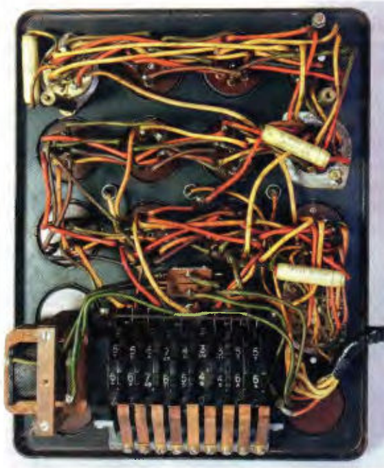
Photo 9: The inside of the socket panel of the Valve Tester. The wiring is quite busy, but the good news is that it rarely goes wrong. Note the copper-plated springs used to create the detents on the thumbwheels.
