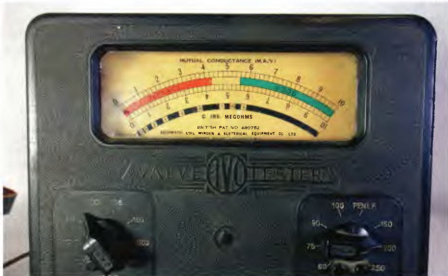
Photo 8: The meter scale on the original AVO Valve Tester. The 0-10 scale could read out either the g_m directly or a proportional value where 10 represented the expected g_m . Interestingly, valves with a gain as low as 56% of nominal were still considered 'good' – presumably due to the expense of replacing them.
