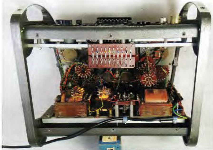
Photo 12: The VCM MkIV is a powerful instrument, but it's challenging to work on because many of the components are packed close together or inaccessible.
