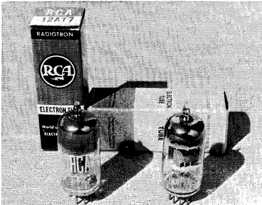
The RF-1 uses two valves: a 6AN8 and a 12AT7. Although the originals tested OK, they were replaced as part of the restoration procedure.
