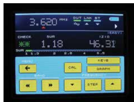
PHOTO 4: A good SWR at 3620kHz.
