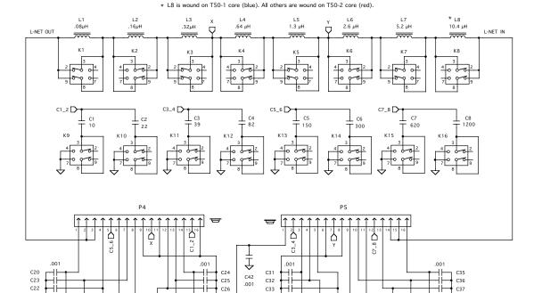
NOTE: K1-K18 are single-coil latching relays, shown in the RESET position. Pins 5 and 6 of each relay are used as tie points but are not internally connected. = On bottom of PC board. All relays on the L-C board are on the bottom.
