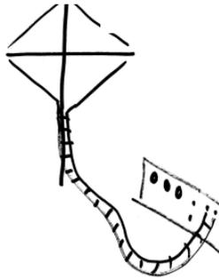
Loops can take on nearly any closed shape such as a square, rectangle, triangle, or diamond shape and they can be fed on the sides or in the corners. The impact of different configurations and feed points is well documented in the many
