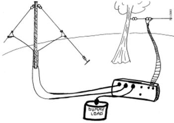
One common benefit of having a switchable antenna controller is the ability to leave a dummy load connected so that you can switch to it conveniently at need.
