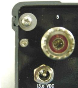
The MAC-200 cover is locked in place with a simple arrangement using an oversized washer to engage a small groove in the side of the cover to prevent its movement. A #4 screw and a slightly oversized washer (#6 or #8) are locked in place by a lock washer to prevent movement of the cover.
