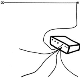
Unbalanced antennas need an RF Ground or counterpoise to create electrical balance and depend on the quality of the ground for a high quality radiated signal. Without a good quality ground, unbalanced antennas will cause interference, lead to RF in the radio room, and be of very low efficiency due to high losses in the ground. Typical unbalanced antennas are long wires and verticals.
