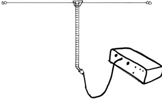
Some antennas, such as the G5RV, use a section of ladder line as a matching device. These transform the impedance of feed point to something near 50 ohms. Usually, the ladder line terminates in a 1:1 balun. The Coaxial line from the transceiver connects to the balun. The MAC-200 can feed this connection directly from one of the coax ports or you can remove the balun run the ladder line directly to the MAC-200 balanced feed line port.
