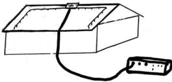
Stealthy antennas are built in a variety of ways. A simple example is a roof-mounted dipole with its ends bent 90 degrees and fed from the MAC-200.
