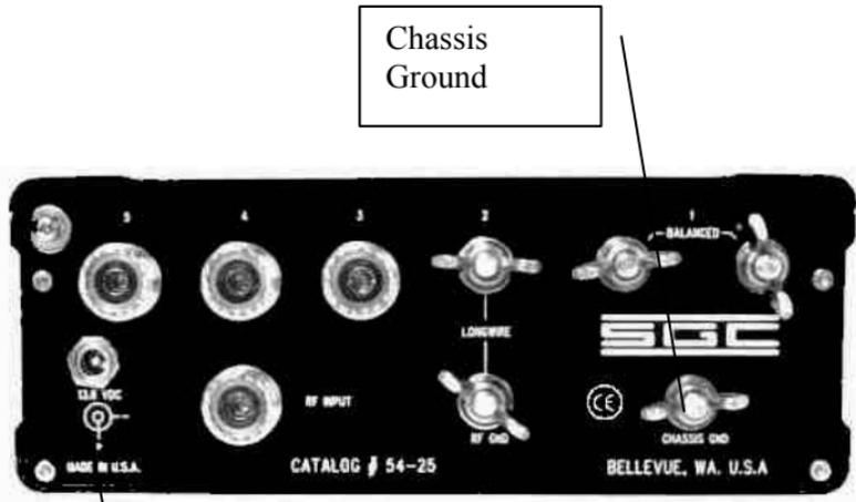
The MAC-200 has a miniature power input jack on the back panel. Any voltage from 10 to 18.5 VDC is suitable for operation. Average current draw will be approximately 230 milliamps. The MAC-200 should be powered from the same power source used to supply your transceiver to ensure that it is energized whenever the transceiver is in operation.
