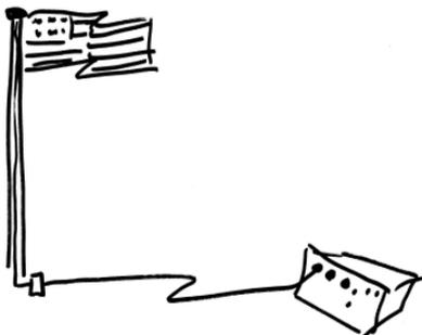
Home made vertical antennas are commonly made in one of two ways. A very common type of construction builds the radial system at the base of the antenna. Flag pole antennas are normally built in this way. Coax line can be run from the MAC-200 to the base of the antenna. The center lead of the coax will feed the radiating
