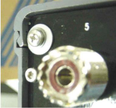
1. Loosen the cover lock on the back panel of the MAC-200 until the washer disengages from the MAC-200 cover.
