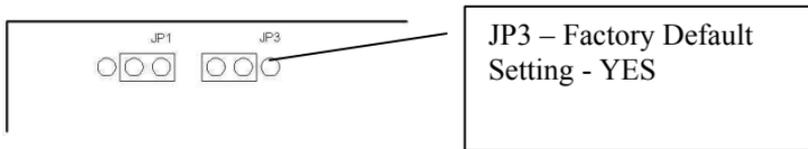
**YES** - In this position the coupler will recall data previously saved and try this data before attempting to re-tune. If the data is valid and the VSWR is less than 2:1 the tune is completed. In this position the coupler will save any new data in its memory for any frequency. A new frequency must first be learned, while in this mode, before it can be recalled.
