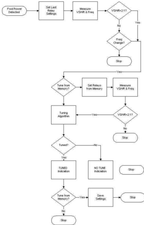
A tune-up algorithm implements antenna matching. It is designed using the MC68HC711E9 microprocessor that features a versatile instruction set, RAM, and EEPROM (memory which is saved after the coupler is turned off).
