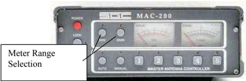
The meter range selection is made on the two push button switches to the left of the meters. Press the switch labeled 20W to activate a 20 watt range. Press the switch labeled 200W to activate the 200 watt range. No harm will come to the meters if the wrong range is activated for the power applied. When a given range is selected, a small LED will light above the switch to indicate which range is currently selected.
