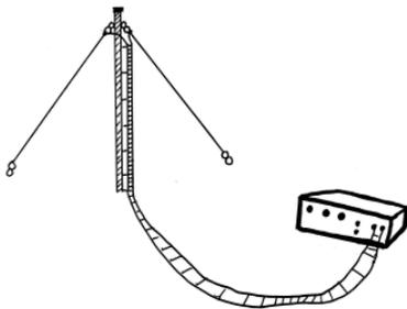
The inverted-V antenna can be fed with ladder line run from the balanced line connection on the MAC-200, but it is also commonly fed from coaxial cable with the center conductor to one side and the shield to the other.
