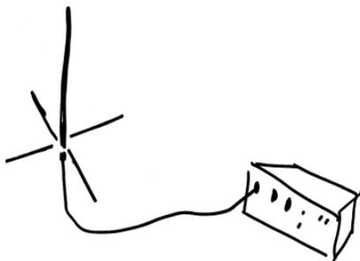
A vertical antenna may be connected to the MAC-200 in a number of ways. Most vertical antennas will require an RF Ground system to function properly, but this may be incorporated into the design of the antenna itself.
