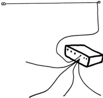
Long wire and inverted L antennas are unbalanced antennas. They are fed from the upper LONGWIRE connection directly with a single wire.
