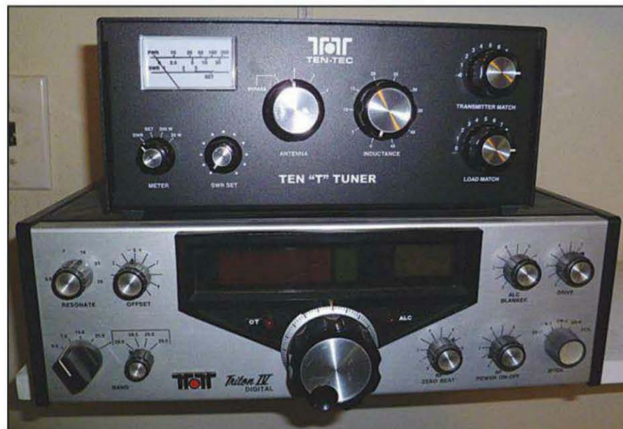
The Ten "T" Tuner ready to go QRV with my classic Ten-Tec Triton IV transceiver.
