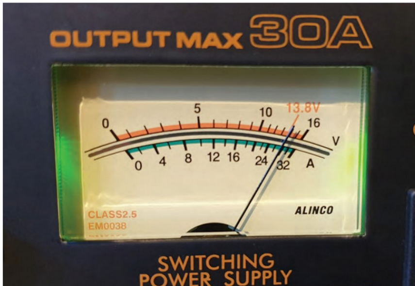
Front panel meter showing the supplied voltage and current.
