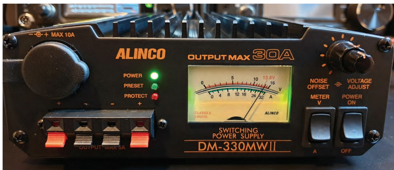
The front panel of the Alinco DM330MW UK MkII, a well-built power supply.
