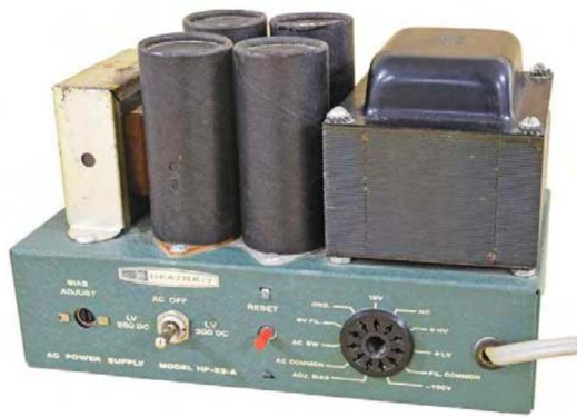
Figure 9 — The HP-23A was produced in the late 1960s and early 1970s to power Heathkit's SB and HW series transceivers. The power transformer is on the right and a filter choke is on the left. The four black electrolytic can capacitors in the middle will be replaced.
