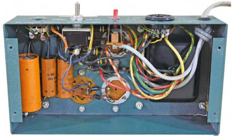
Figure 10 — The Hayseed Hamfest full kit includes three electrolytic capacitors to replace the ones on the left side, underneath the chassis.
