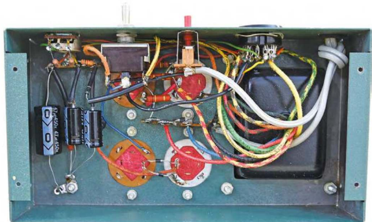
Figure 12 — Inside the rebuilt HP-23A, the modern electrolytic capacitors, metal film resistors, and 1N4007 rectifiers take up a lot less space than the original components from 50 years ago.
