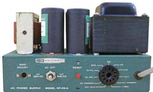
Figure 11 — The HP-23A power supply with the Hayseed Hamfest can capacitors installed retains its original appearance. The new capacitors are an exact fit where the old ones were removed.
