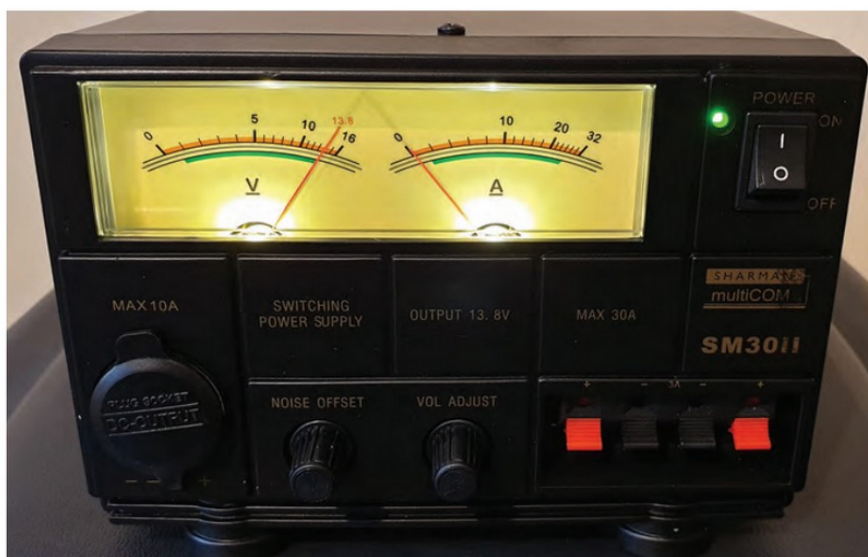
The front of the Sharman multiCOM SM-30II switch-mode power supply unit.
