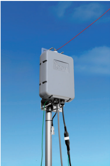
Long wire antenna
