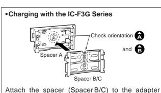
(Spacer A) with the orientation as illustrated in the diagram above.
