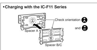
Attach the spacer (Spacer B/C) to the adapter (Spacer A) with the orientation as illustrated in the diagram above.
