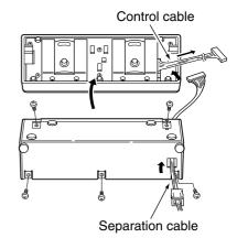
⑦ Remove 2 screws from the cable hole cover on the linear amplifier rear panel. Insert the separation cable into the cable hole. Keep the hole cover and screws for future use.
