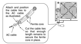
**NOTE:** Only one ferrite core is attached with the IC-PW1EURO.
