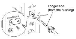
(8) Plug the other longer end (from the bushing) of the separation cable into J10 on the JACK unit through the cable hole. Connect the control cable to J11.
