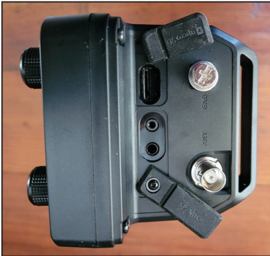
Photo B. The right and left sides of the radio contain multiple jacks for the mic, key, external power, etc. Note rubber plugs that seal the jacks when not in use.
