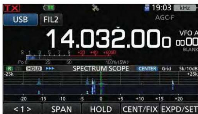
Figure 2 — The IC-705 spectrum panadapter display, showing activity on 20 meters.
