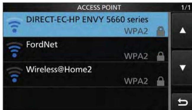
Figure 5 — You can connect the IC-705 to a wireless network for remote control via the internet. It's simply a matter of choosing the desired network and entering the password.
