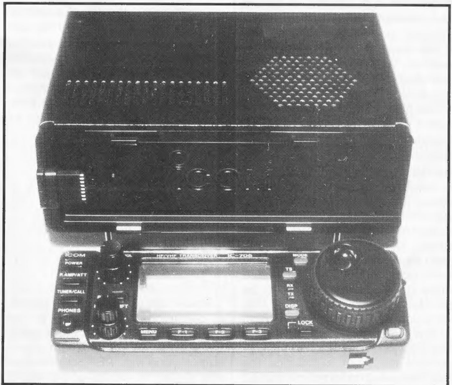
The detachable front panel disconnected from the IC-706.
