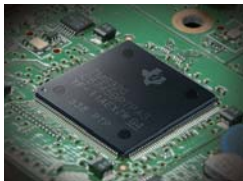
32-bit floating point IF DSP
