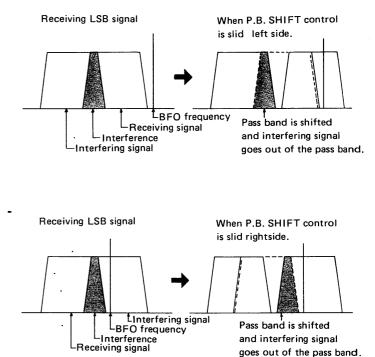
When the optional crystal filter, FL-30, is installed, the Pass-Band Shift system will be changed the Pass-Band Tuning system.
