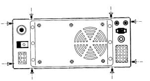
2. Remove the eight screws at each end of the rear panel.
