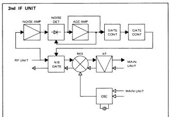
During receive, the 39MHz signal from the RF unit is fed to the 2nd mixer which is a high level DBM, and mixed with 30.72MHz 2nd local oscillator signal to convert it in 9.0115 MHz 2nd IF signal.
