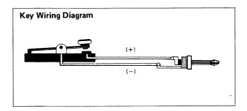
If the terminals have polarity, be sure to make the correct connection. Note that the keyed voltage when switching with semiconductors or relays with resistors in the circuit, should be adjusted to be below 0.4 Volts!
