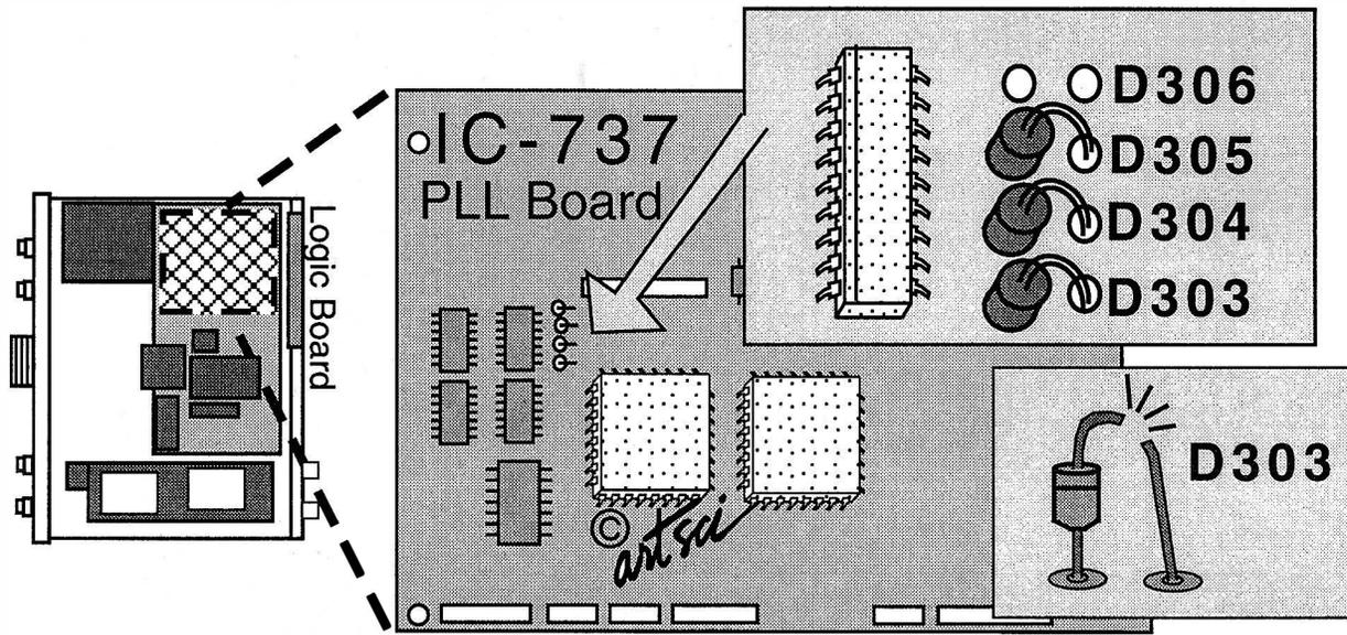
Note: Accessing the PLL Board may require taking out many of the other components of the radio.
