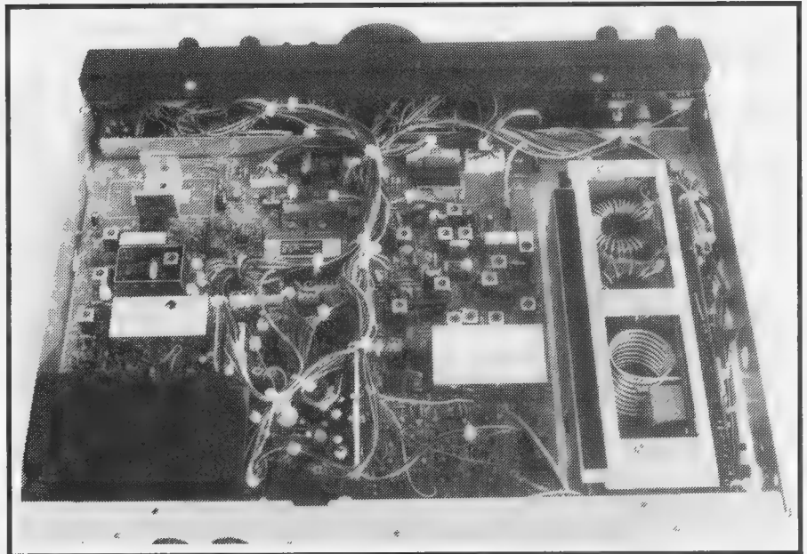
The main circuit board of the IC-737 with the bottom cover removed. The bracket at the top left takes the 455 kHz CW filter. Both CW filters plug in, soldering not needed.
