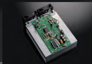
PA Unit with a Large Heatsink
