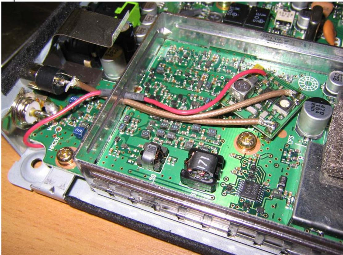
Red lead is power taken from the DC input to the ICOM. Circuit board is grounded and held by 3 vero pins that are soldered through the circuit board. This required a drill to enlarge the holes.
