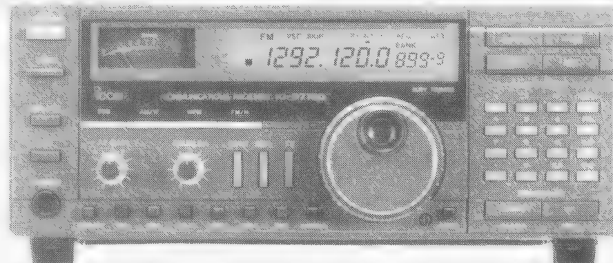
The versatile ICOM IC-R7100 VHF/UHF All-mode Communications Receiver.
