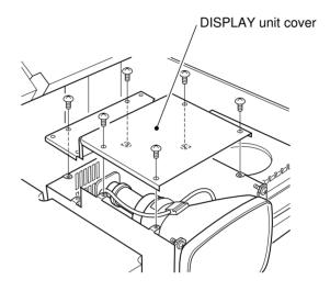
⑥ Remove the 4 screws and 2 connectors from the DISPLAY unit (CRT) and remove the unit as shown in the diagram below.
