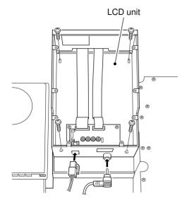
® Replace the rubber spacer from the backside of the front panel with the supplied one. Take care of the direction.
