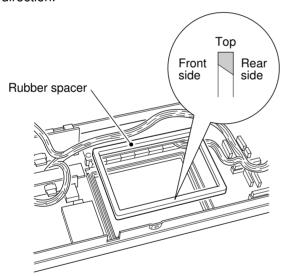
Remove the 4 screws from the front panel and replace the CRT screen filter with the LCD screen filter as shown in the diagram below. Assemble the front panel.
