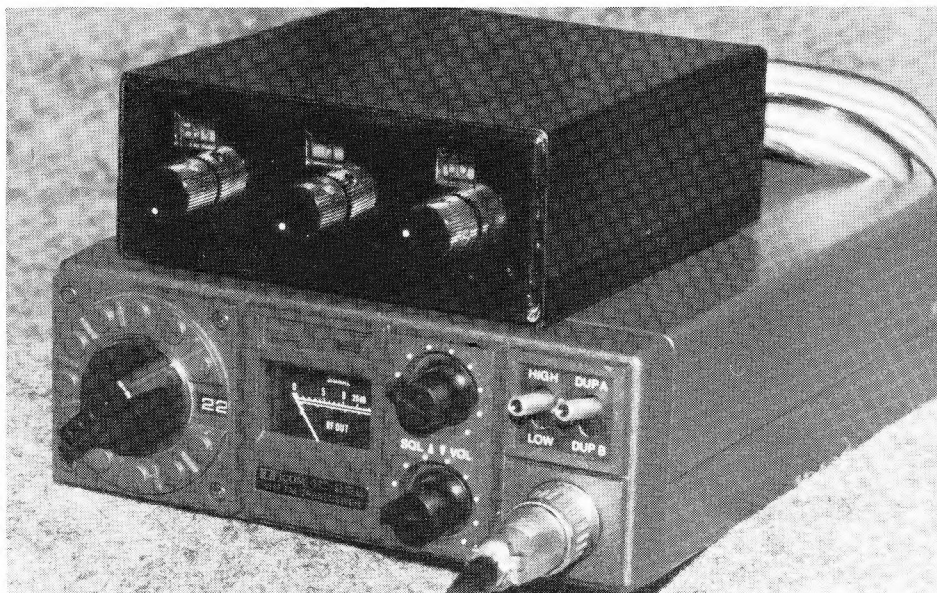
IC22S with Home Brew Channel Synthesiser.
