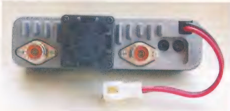
Photo 5: View of the rear of the main body of the transceiver. The antenna socket at the left is the main Tx/Rx antenna. The cooling fan is obvious. The centrally located antenna socket is for "Diversity Reception" (see text). The two small sockets near the DC lead at the right hand side are the two external speaker sockets.
