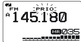
Pauses on a memory or call channel when a signal is received.
