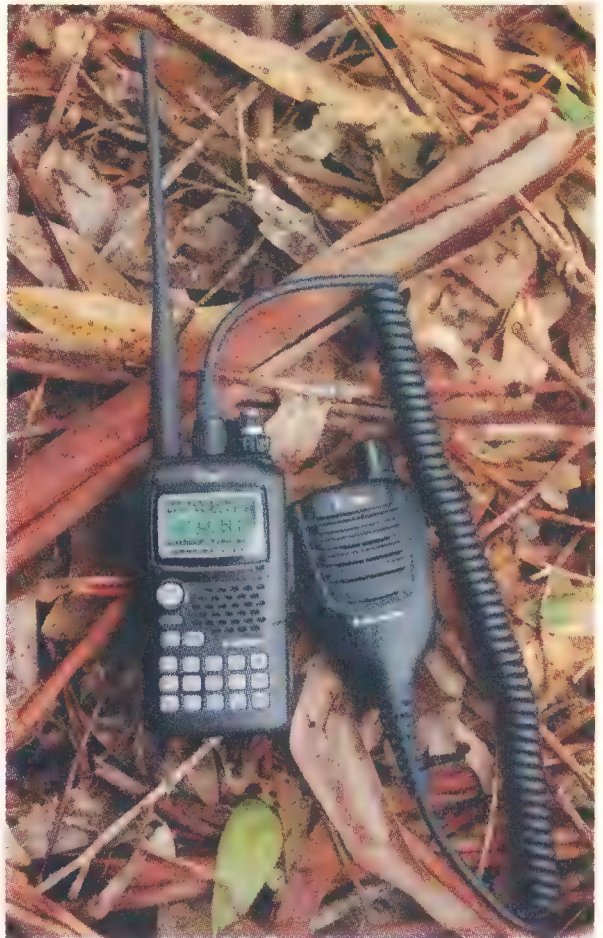
Photo 2: The IC-92AD and optional HM-175GPS displaying the current position using the GPS-A function. No need to worry about dampness or rain drops with this radio, rated waterproof to 1 m depth for up to 30 minutes.
