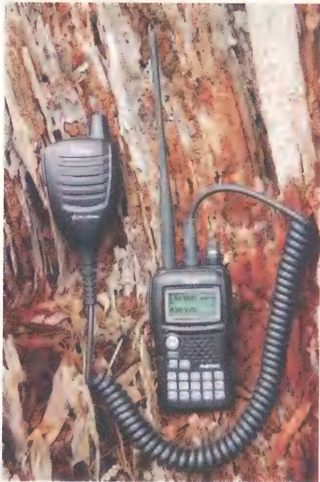
Photo 1: The IC-92AD and optional HM-175GPS, with the display in "dual watch" mode.
