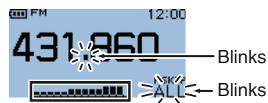
The S-meter shows the received signal strength.
