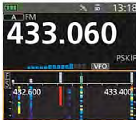
Figure 2 — The ID-52A's color waterfall display is a unique feature. Your receive frequency is indicated by the red line.
