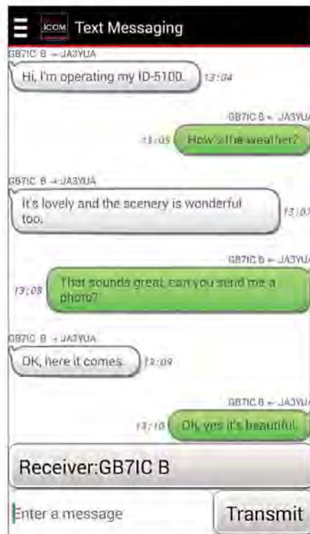
Figure 3 — If you own an Android or Apple mobile device, the RS-MS1 remote control software will use the ID-52A's wireless Bluetooth connection to do all sorts of clever things, such as exchange text messages in the D-STAR mode.
